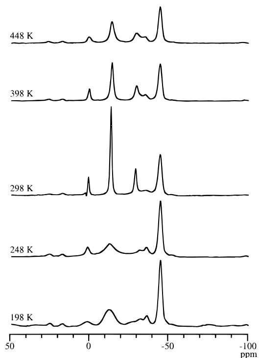
Figure 2. 80.8 MHz variable-temperature ^{31}\text{P} MAS Bloch decay spectra of a SPA sample evacuated at 373 K for 2 h. Phosphoric acid (ca. 2 ppm) and oligomerized acids (–12 and –24 ppm) are in a glassy state at 248 K and below, and in a solution state at higher temperatures. Broadening at the highest temperatures studied may reflect chemical exchange. All spectra are the result of 12 transients utilizing a 60 s recycle delay and a spinning speed of 5000 Hz.
